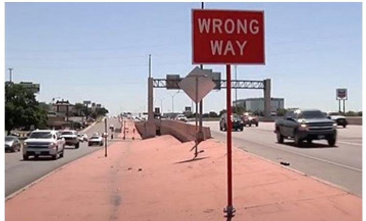
As a countermeasure, red reflective tape can be seen running down the entire length of the Wrong Way sign.
